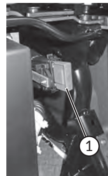
Main fuse for leisure battery
